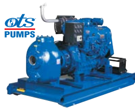
O Series® Engine driven Size: 4" (100 mm) Power: Deutz - Diesel Max Capacity: 730 GPM (46.1 lps) Max Head: 280' (85.3 m) Materials of Construction: Copper Alloy, Aluminum or Cast Steel Housing
