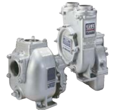
O Series® Power take-off or hydraulic motor driven Size: 2" (50 mm) to 3" (75 mm) Max Capacity: 400 GPM (25.2 lps) Max Head: 440' (134.1 m) Seal Elastomer: Viton® Materials of Construction: Copper Alloy, Aluminum or Cast Steel Housing
