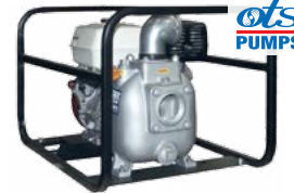
O Series® Engine driven utility Size: 3" (75 mm) Power: Honda - Gasoline Max Capacity: 400 GPM (25.2 lps) Max Head: 160' (48.8 m) Materials of Construction: Copper Alloy, Aluminum or Cast Steel Housing
