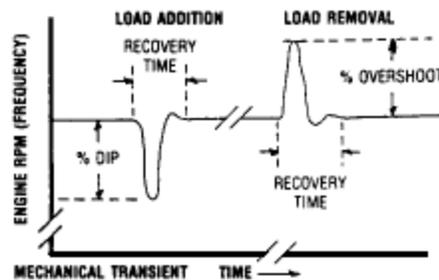
Transient response is measured by percentage frequency change and duration (see Figure 1). The amount of time it takes for the engine to return to steady-state operation is called recovery time. This can vary from as little as 1 second to 20 seconds. In general, the greater the load added to the bus, the greater the percentage of dip and the longer it will take the engine to recover.
